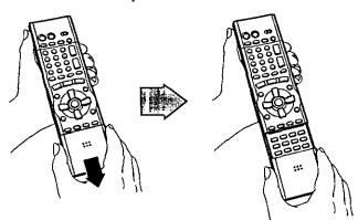
Hold both sides of the remote control's cover to open it. (You can also open it by pressing on the center of it and sliding it down.)
